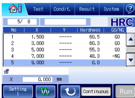
This view is used for the Jominy test or similar applications. The multi-point screen features a navigation function that guides the user to the test position.
