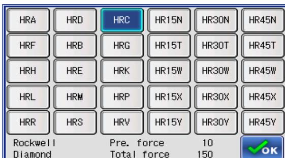
Directly select the required hardness scale from the menu and have full control over the time cycle settings.
