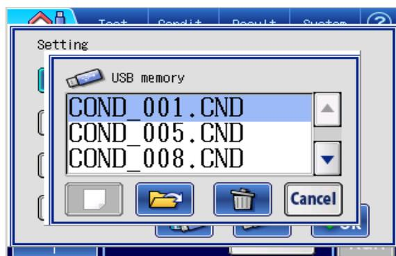
Time-saving storage of user-defined test setups. Test condition files can be stored on a USB memory drive. Conditions can also be set directly from a condition file on the USB stick.
