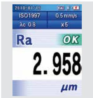
Parameter display Ra with tolerance evaluation
