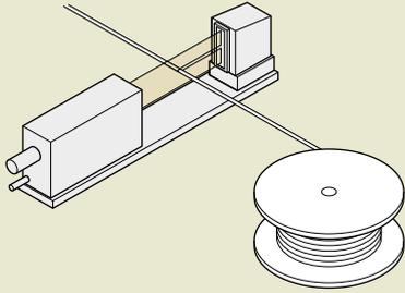
**Measurement of outer diameter of cylinder**
