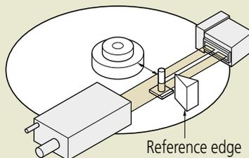
**Measurement of gap between rollers**
