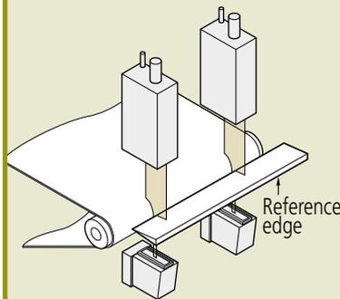
**Measurement of spacing of IC chip leads**
