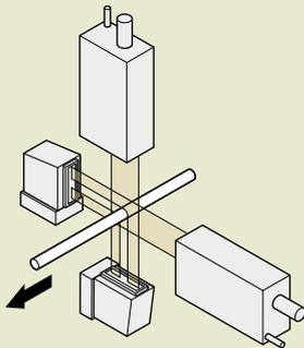
**Measurement of thickness of film and sheet**
