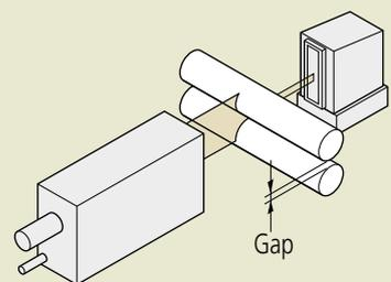
Measurement of tape width
