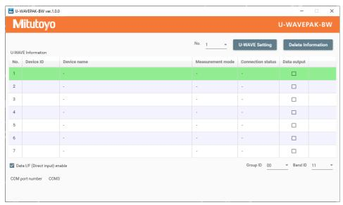
(2) The maximum number of units of U-WAVE-TCB/U-WAVE-TMB to be set up is seven. To set up a U-WAVE-TCB/U-WAVE-TMB, click on a number in the table [U-WAVE Information]. You can also select a number from the drop-down list at the top-right of the window.
