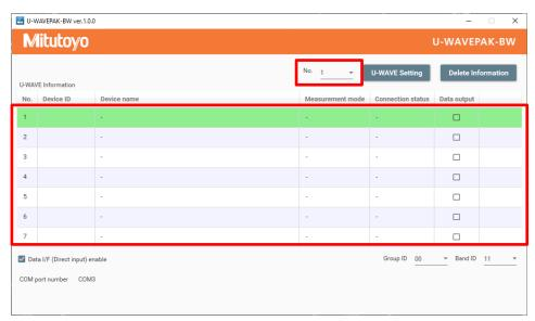
(3) Click on the [U-WAVE Setting] button to open the setting window.
