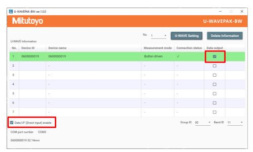
(3) When you wish to input measurement values in an Excel spreadsheet, activate cells in the spread sheet, and then send the measurement values from the U-WAVE-TCB/U-WAVE-TMB with the keyboard input mode enabled.
